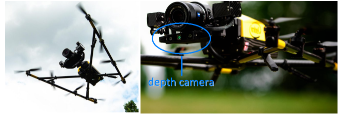
Figure 2. Drone with depth sensor
