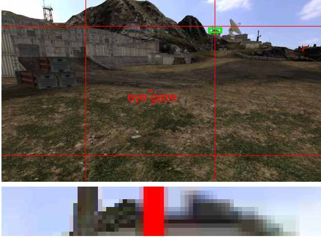
Figure 3. Foveated compression. Top: the center area around the eye gaze is compressed in original resolution, while the eight other areas have been resized by 2x in each dimension before compression. Bottom: close-up on the green marked rectangle, showing on the left the high resolution image while on the right the area with reduced pixel size is shown, upscaled with bilinear filtering on the GPU.
