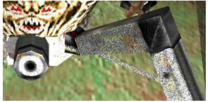
Figure 6. Epsilon issues during casting a shadow ray. The ray self-intersects with the surface to be shaded and produces a flickering moiré pattern.
