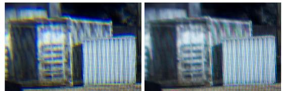
**Figure 8:** Seen through the lens of the Oculus Rift. Left: no handling of chromatic aberration. Right: chromatic aberration minimization enabled.
