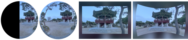
Figure 2: Left-to-right: 180^\circ \times 180^\circ image on a half sphere, 360^\circ \times 180^\circ image on a full sphere, regular image on a flat canvas, cylindrical panorama on a curved canvas.
