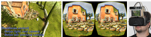
Figure 3: Left: image created for the outside screen. Center: lens distortion compensated stereo image for the inside viewer. Right: photo of the HMD prototype 2.
