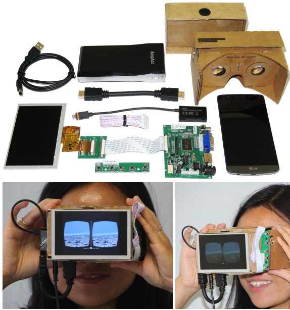
Figure 2: HMD prototype 1. Google Cardboard extended with a front-facing screen that duplicates the internal image.
